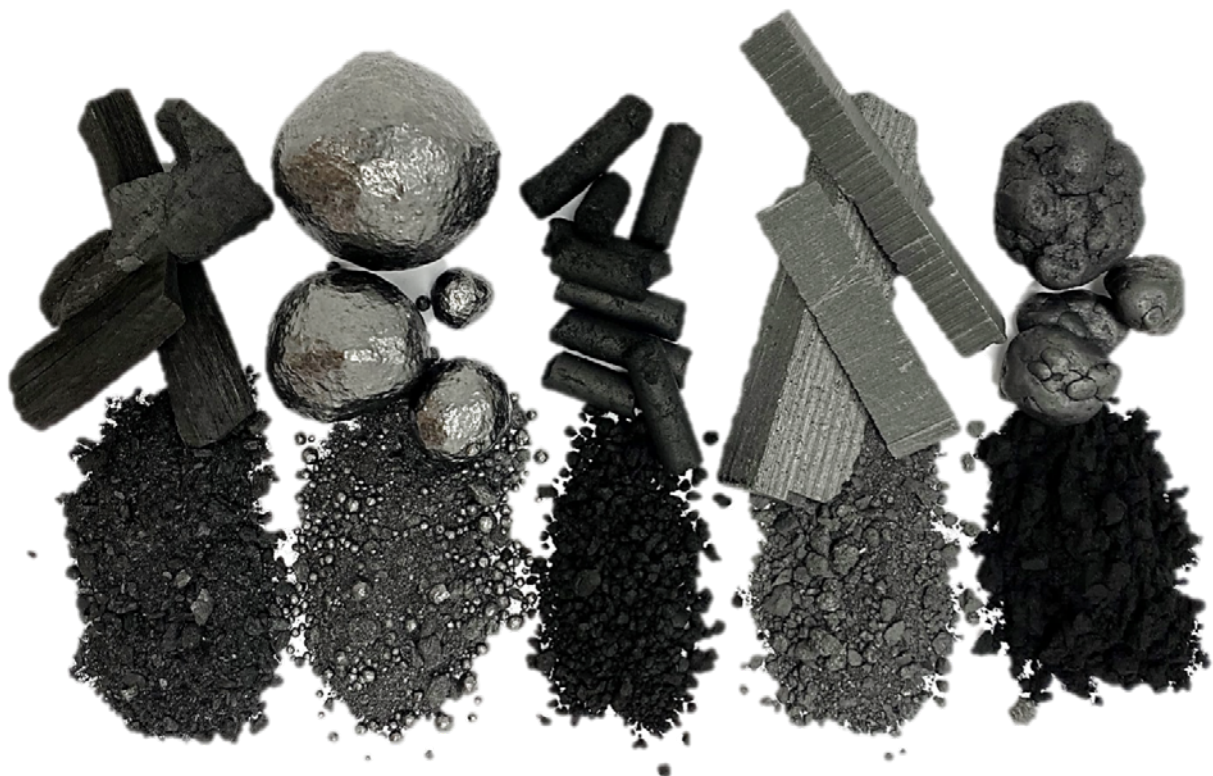
f.l.t.r. charcoal, carbon agglomerates, soot coke pellets, graphite blocks, graphite mixture
